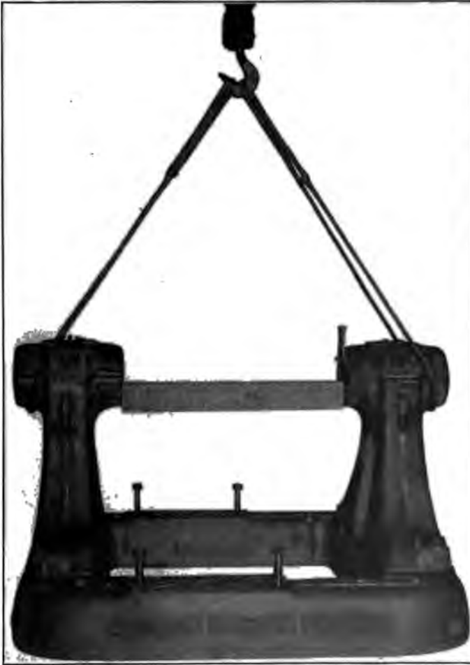
FIG. 32.—Method of lifting base and standards.
